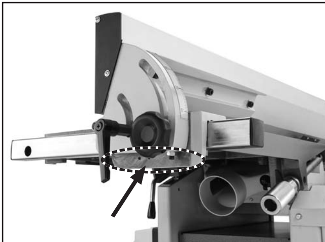
Figure 8. Outside fence lubrication location.
